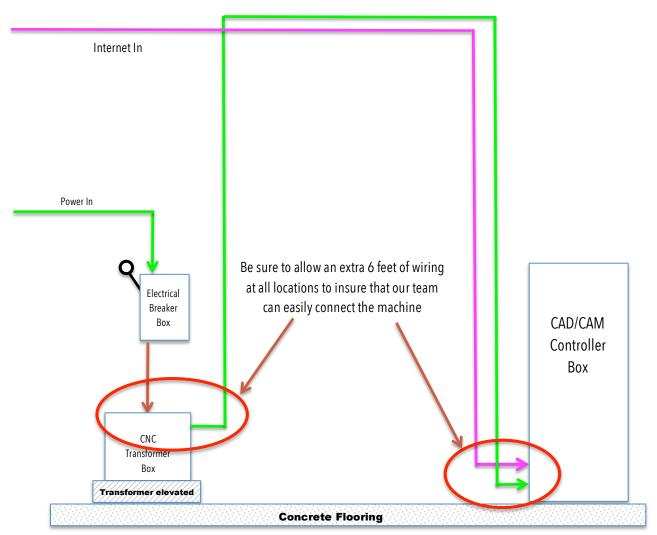
CNC Connection: #6 copper wire – gauge required throughout connection including ground
