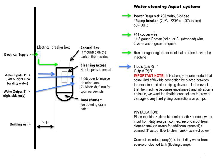
Be sure to prepare your installation location with these fittings that will couple and fit perfectly with our machine fittings. These elements are what you should have in place.
